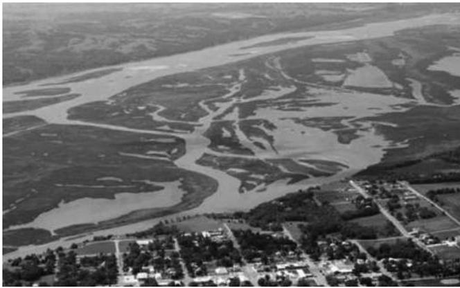
**Fig. 4.** Deltaic deposits in Lewis and Clark Lake near Springfield, South Dakota (reprinted from Missouri Sedimentation Action Coalition 2012, with permission)
