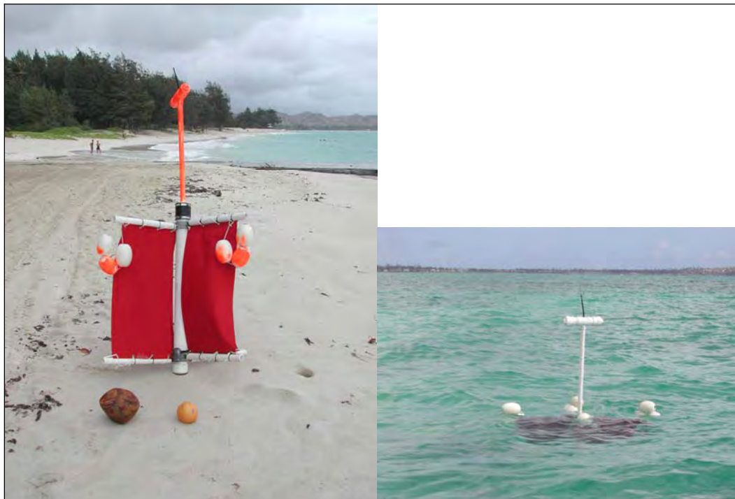
Figure 5. GPS current drogue (left) with traditional drifter (behind grapefruit) and Hawaiian drifter (coconut). Drifter floats just below surface (right).
