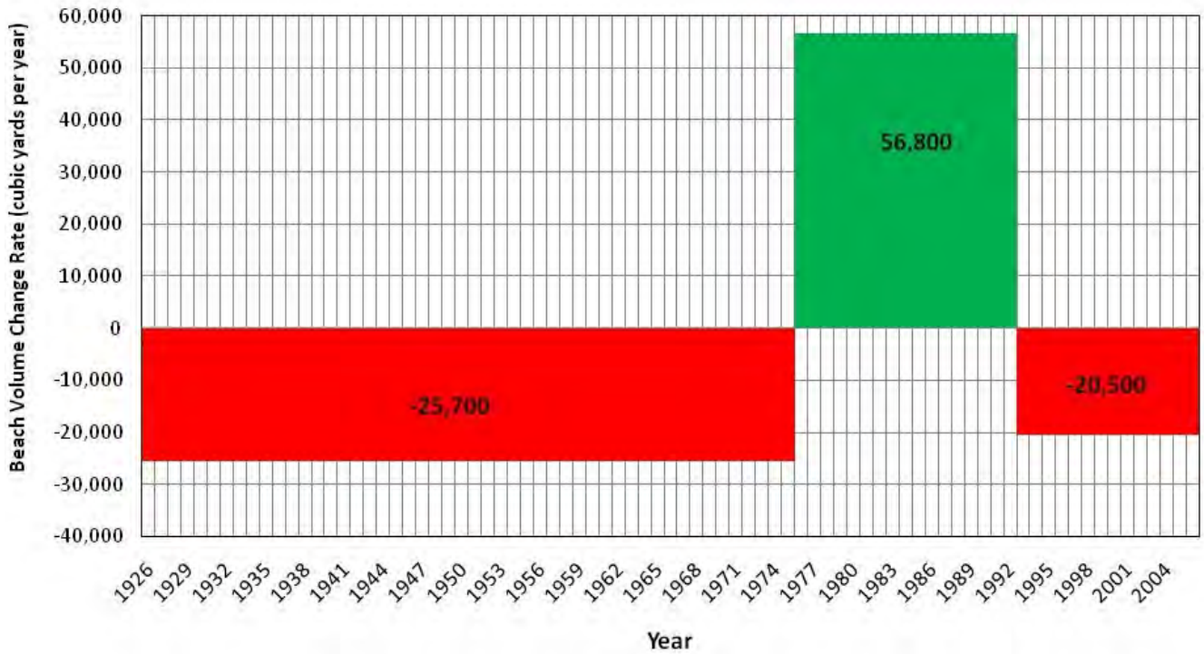
Figure F-7. Historical Beach Volumes / Change Rates for Kekaha Beach Littoral Cell
