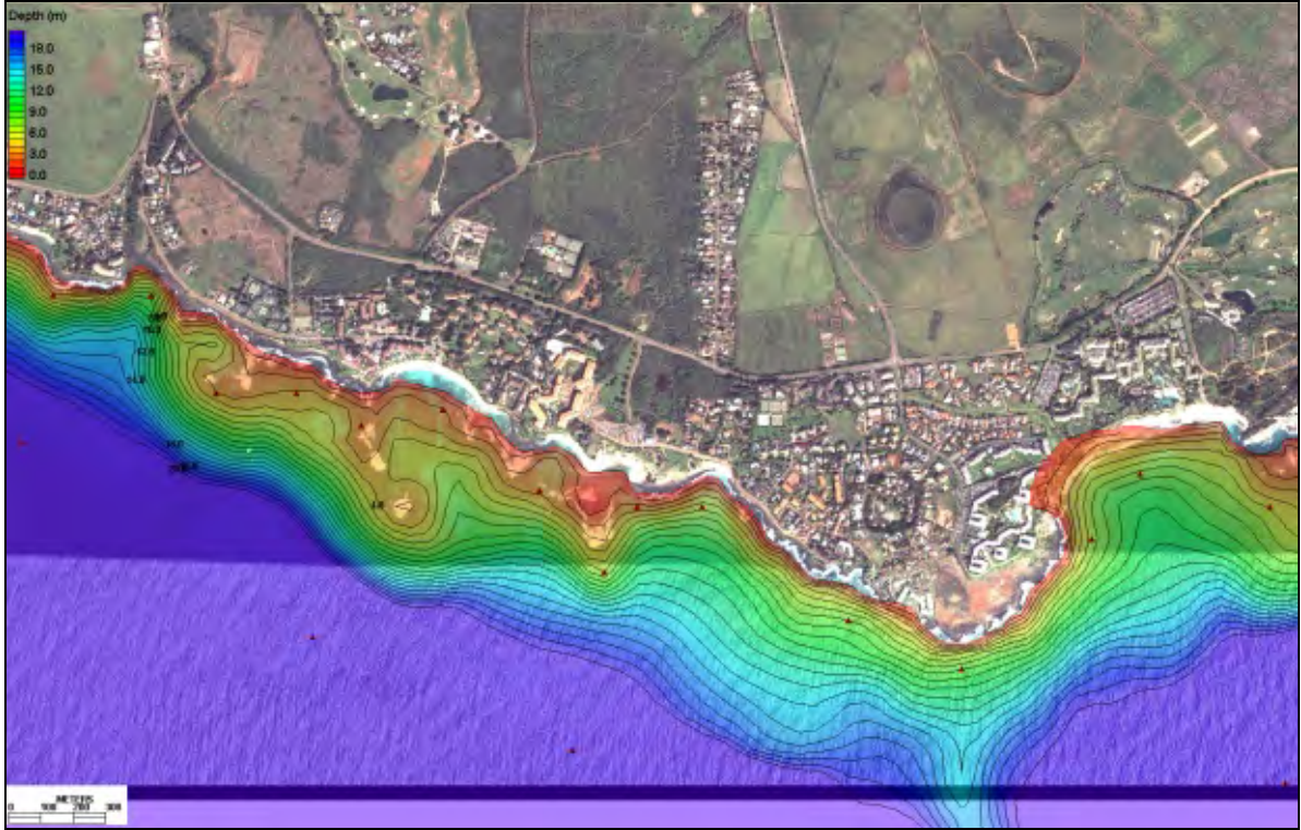
Figure C-27. STWAVE Nearshore Grid Adjacent to Poipu Beach in Poipu Region (1m contours shown)
