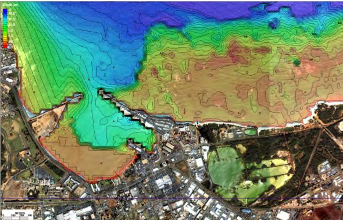
Figure B-28. STWAVE grid adjacent to Kahului Harbor in Kahului Region (1-meter contours shown)
