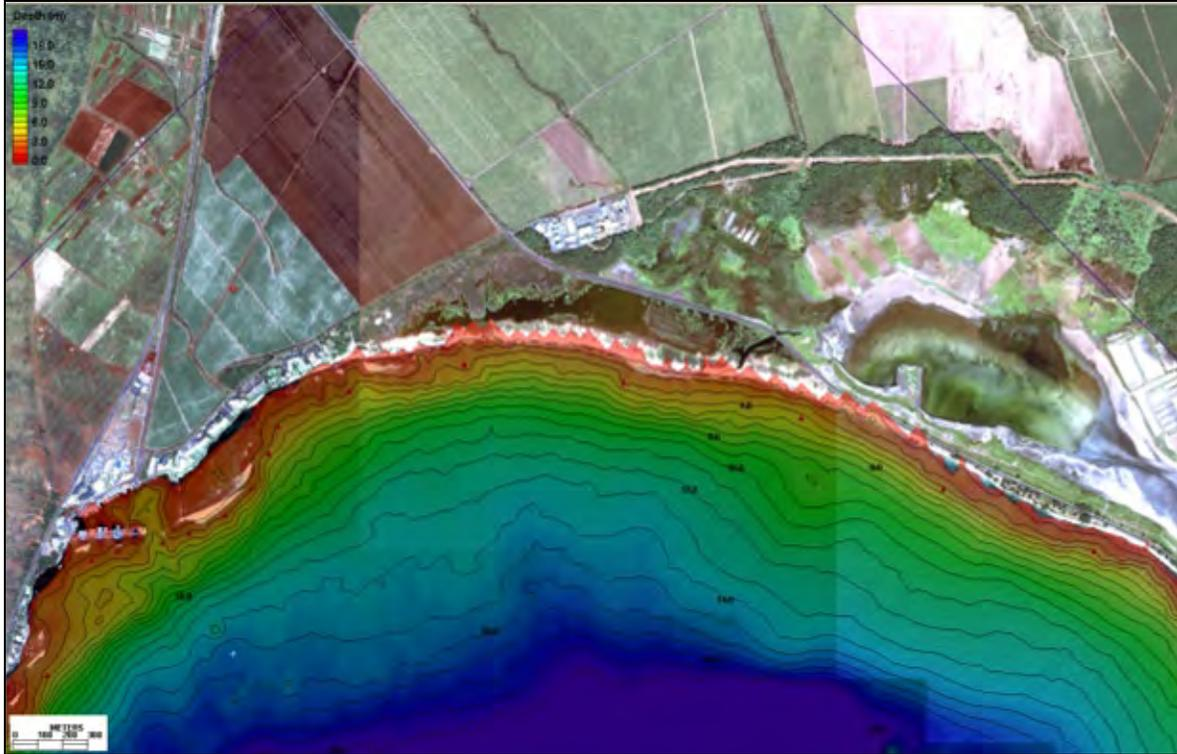
Figure C-28. STWAVE Grid Adjacent to Maalaea Harbor in Kihei Region (1-meter contours shown)
