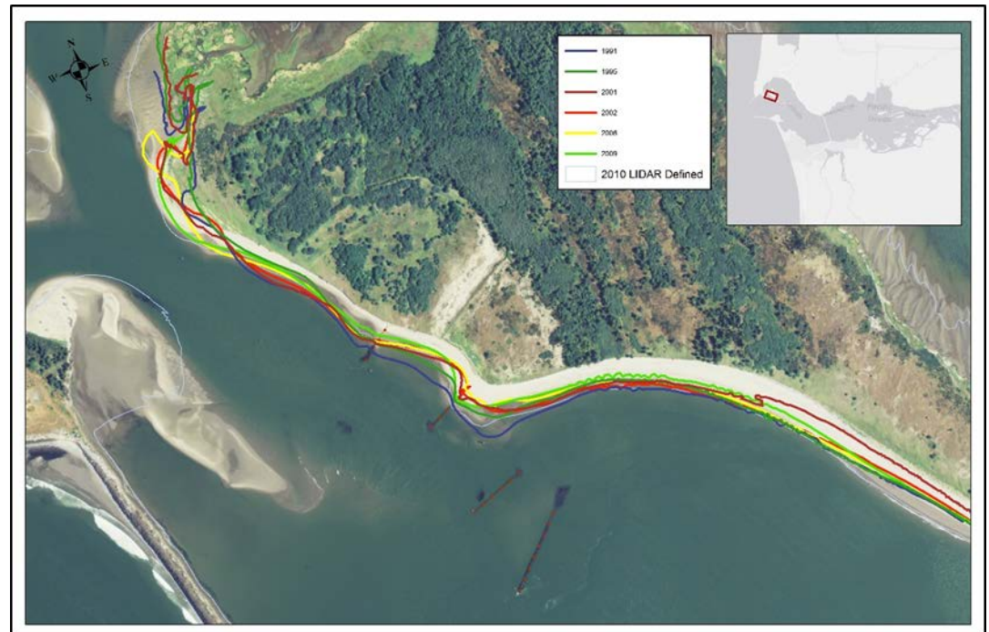
West Sand Island – Historical Photogrammetry of Shoreline Movement
