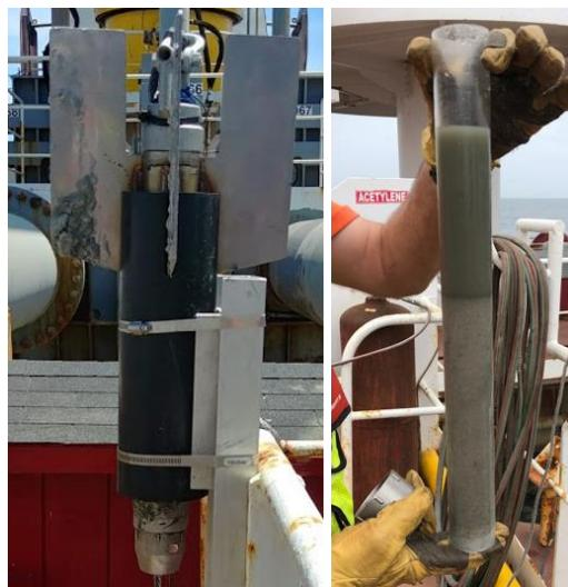
Sampling from the hopper to determine fines content of the loaded dredged material
