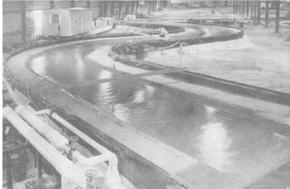
Figure 1. ERDC (WES) “Curved Channel Model” used to develop classic equations to compute influence of curvature on riprap size.
