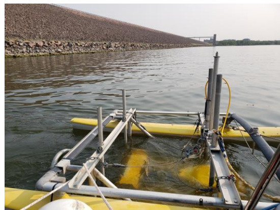
Figure 2: Chirp sub-bottom profiler collecting data at Cherry Creek Reservoir, CO.
