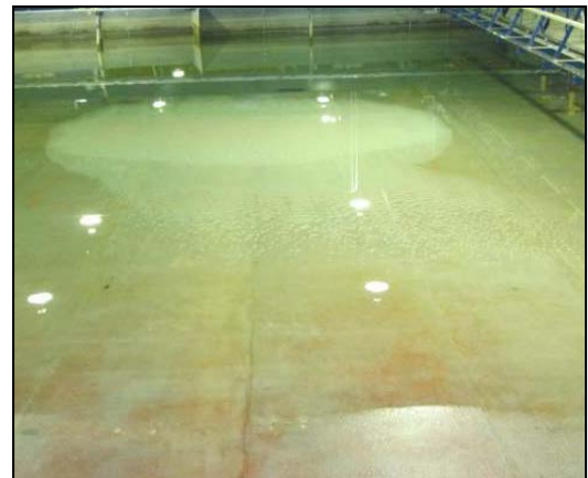
LTSF is employed for study of mixed sediment nearshore berm transport
