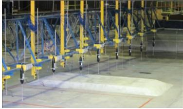
hemisphere capable of simulating an infinite shoreline. The LSTF can produce large-scale laboratory waves, pump and recirculate longshore current, measure the quantity of sands that moves along the beach, and contains a fully programmable instrumentation bridge and data acquisitions system.
