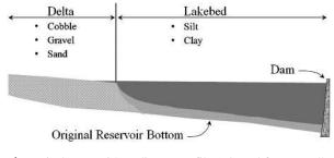
**Fig. 1.** Typical reservoir's sediment profile (adapted from Randle and Ferrari 2010)
