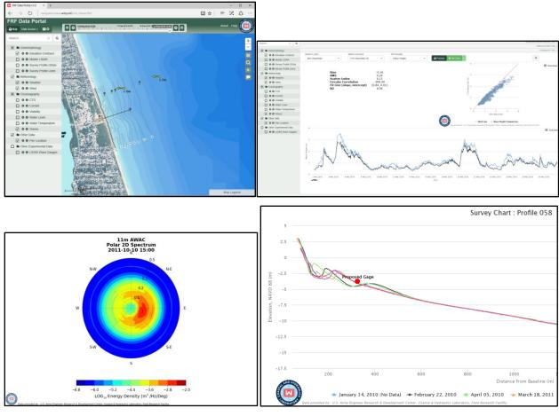
FDIF – Data Portal Version 1.0 (top left), comparison tools - displaying observations from 17 & 26m waveriders along with error statistics (top right), plotting tools - displaying polar 2D wave spectrum from 11m AWAC wave and current sensor (lower left), and profile tool – displaying selected surveys along a transect north of the pier (lower right).
