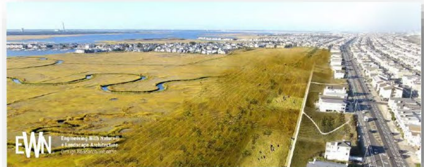
Restored wetland integrated into a "horizontal" levee provides flood risk reduction, sea level rise resilience, environmental, and social value
