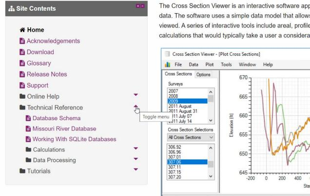
The Cross Section Viewer is an interactive software application for managing and visualizing river transect data. The software uses a simple data model that allows most types of transect data to be stored and viewed. A series of interactive tools include areal, profile and longitudinal plots as well as several geomorphic calculations that would typically take a user a considerable amount of time to produce.
