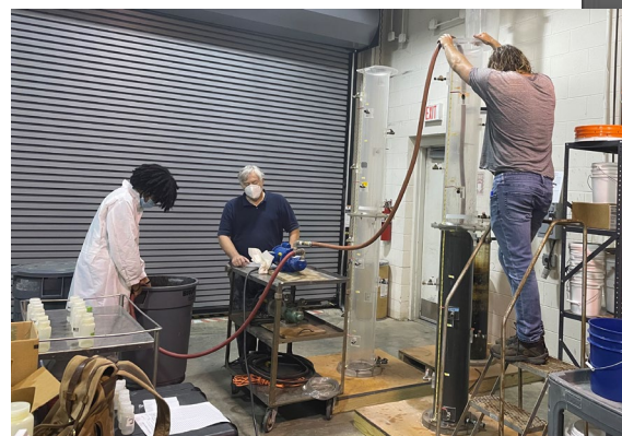
Column Settlement Testing
