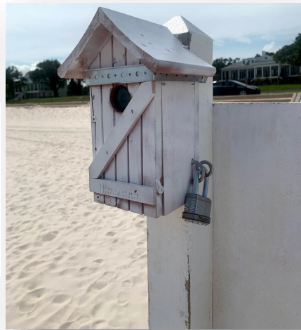
Time-lapse camera disguised as a birdhouse for theft- avoidance
